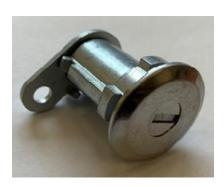
If the lock uses RA4 / 1970AM single sided key (B&S Groove 60) with 1 inch diameter face cap: D-43-204 - single door lock coded with spare face cap for rekeying and reversible pawl for right or left side (NOTE: to use this lock on the baggage compartment door the original pawl must be reused.)
